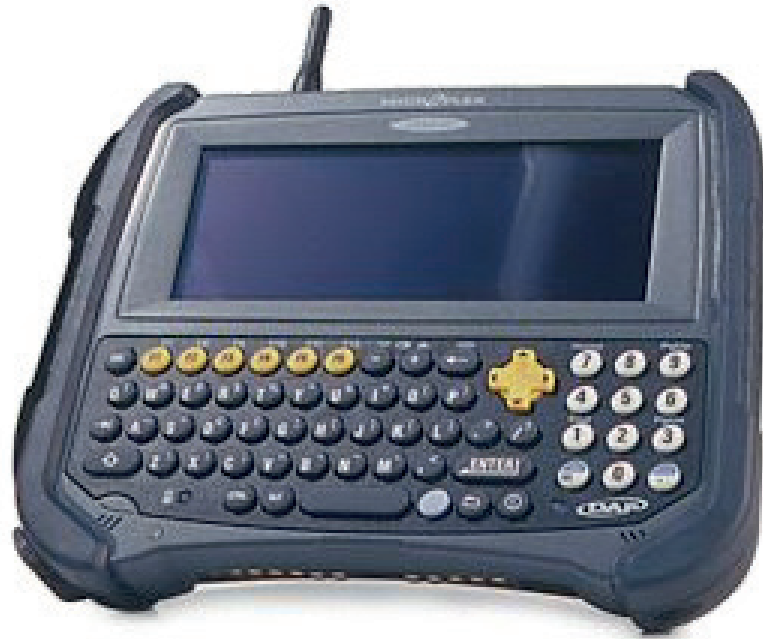
Figure 2: A mobile data terminal in a police patrol car receives instructions from a CAD system via UHF Radio
