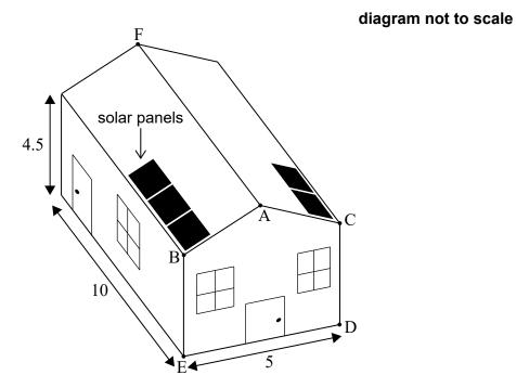
Each panel is 1.6 m long and 0.95 m wide. All the panels must be arranged in uniform rows, with **the shorter edge** of each panel parallel to AB or AC. Each panel must be at least 0.3 m from the edge of the roof and the top of the roof, AF.
