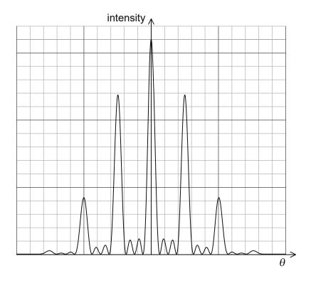
The number of slits is increased keeping the width and the separation of the slits unchanged.
